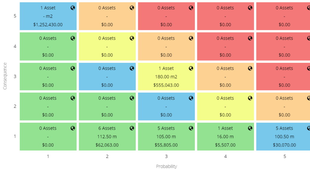
Figure 17: Bridge & Structural Culvert Risk Matrix
